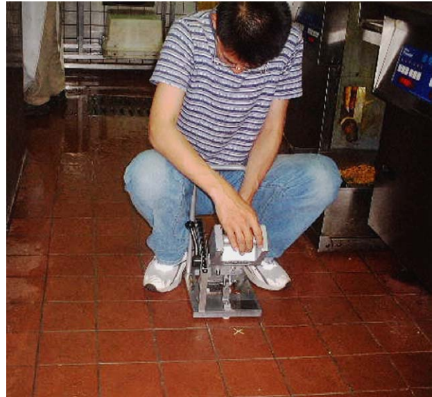
Fig. 1. Measurement of friction coefficient using the Brungraber Mark II slipmeter.
