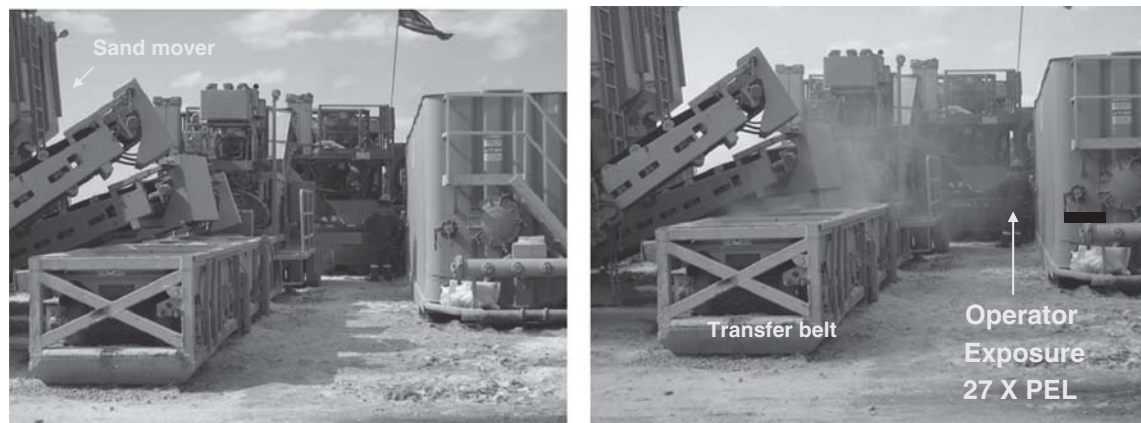
FIGURE 5. Transfer of sand from a sand mover via transfer belt at a hydraulic fracturing drilling site. Exposure to silica measured at 27 times the allowable Occupational Safety and Health Administration permissible exposure limit. Photo courtesy of Eric J. Esswein, NIOSH Western States Office. Reproduced with permission.
