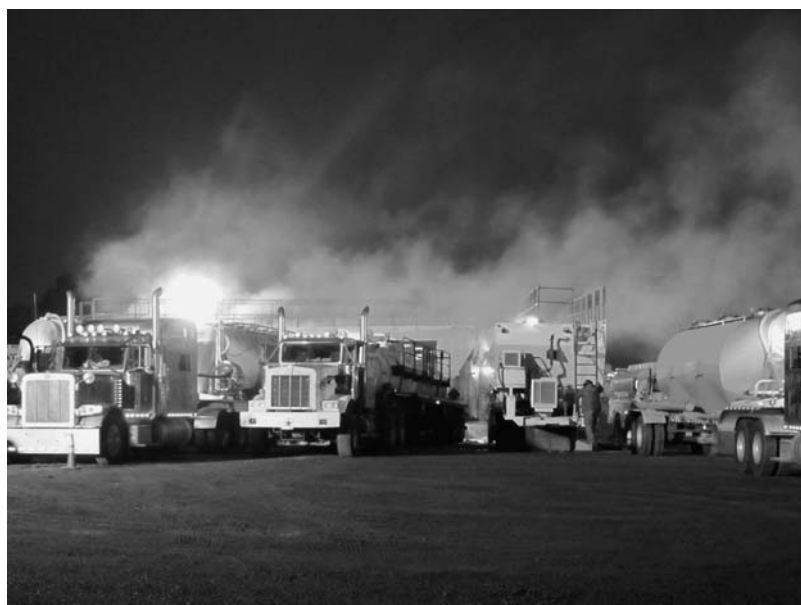
FIGURE 4. Loading sand from sand refill trucks into sand movers at a hydraulic fracture drilling site. Photo courtesy of Michael Breitenstein. Reproduced with permission.
