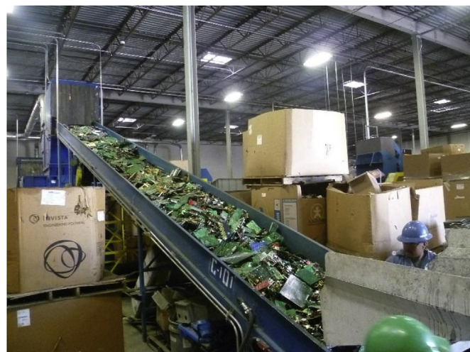
Fig. 1. Electronic shredding conveyor.
