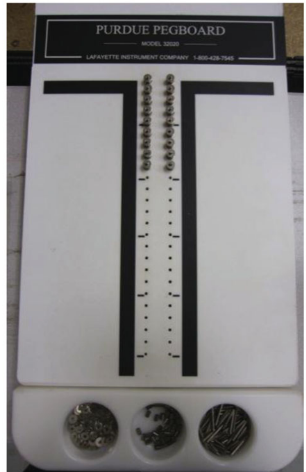
FIGURE 3 Purdue Pegboard Task. Participants assembled pieces (left) into holes in a pegboard (right) (color figure available online).
