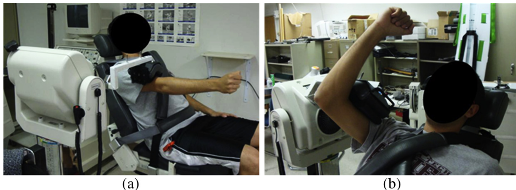
Fig. 1. Arm postures used for strength testing and endurance tasks: (a) extended posture and (b) flexed posture. Note that participants needed to be semi-reclined so that the dynamometer axis of rotation could be aligned with that of the shoulder.
