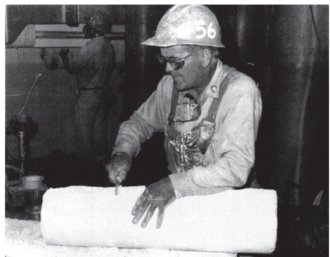
Figure 2. Worker shaping a half-round with a knife, no protective clothing. Photo Source: Carl Mangold. Previously published in Hollins et al., 2009.
