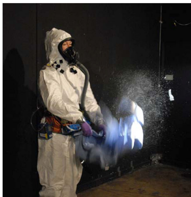
Fig. 1. Depiction of chamber and testing arrangement. Photo depicts person shaking asbestos-contaminated clothing.
