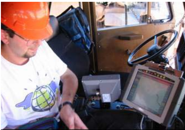
Figure 2: A picture showing the installed rugged flat panel computer CAT 793 truck.
