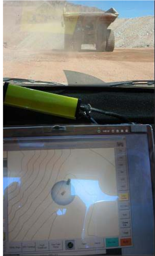
Figure 20: Picture taken at Morenci during the proximity-warning test.
