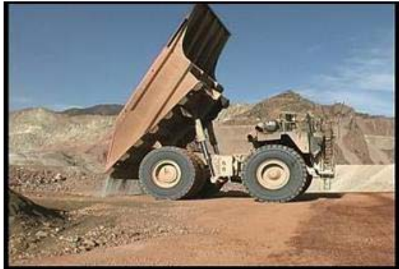
Figure 22: The mine truck during the dumping process based on the new, updated map which was radio transmitted from the dozer
