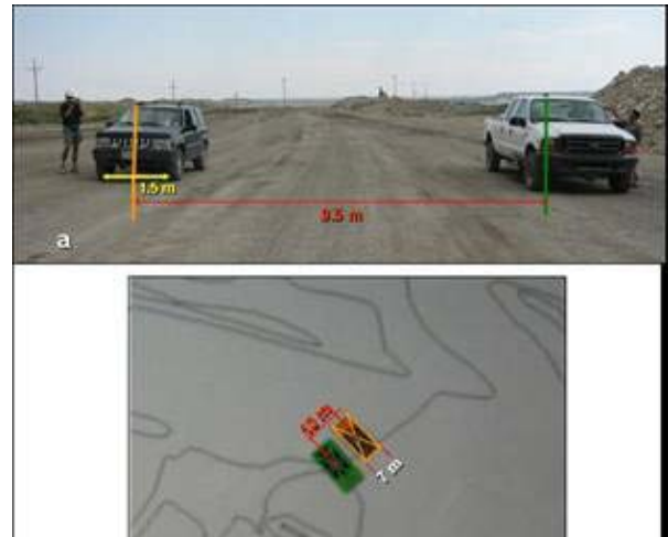
Figure 24 (a-top b-bottom): Measurements to check consistency between VirtualMine models and the vehicles on the actual field.
