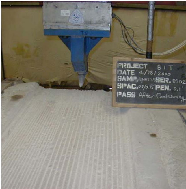
Figure 10: Sample during for linear cutting tests.
