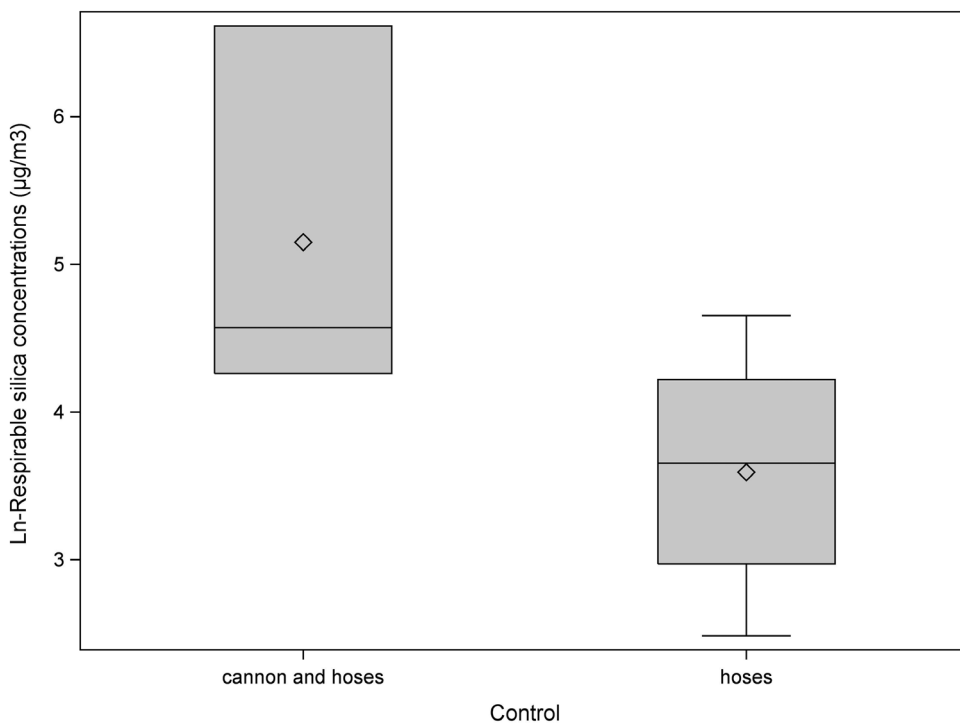
Figure 3. Comparison of area RD concentrations ( \mu\text{g}/\text{m}^3 ) at demolition site A with combination of water cannon and water hoses versus water hoses ( P = 0.03 ).
