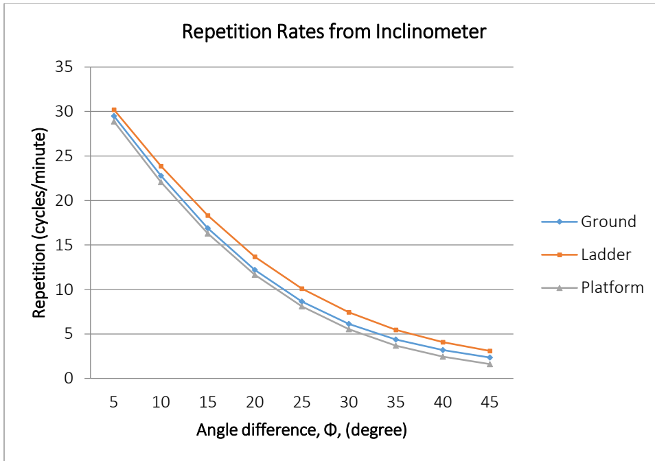
Figure 16 – Mean repetition rates from the accelerometer data using angle thresholds ( \Phi ) between 5° and 45°
