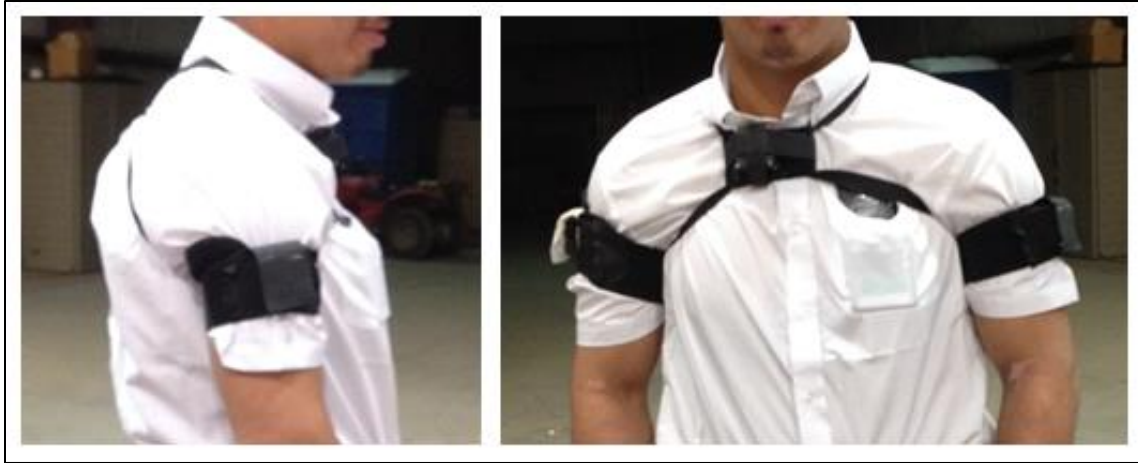
Figure 9 – Upper arm accelerometers: (left) side view, (right) front view
