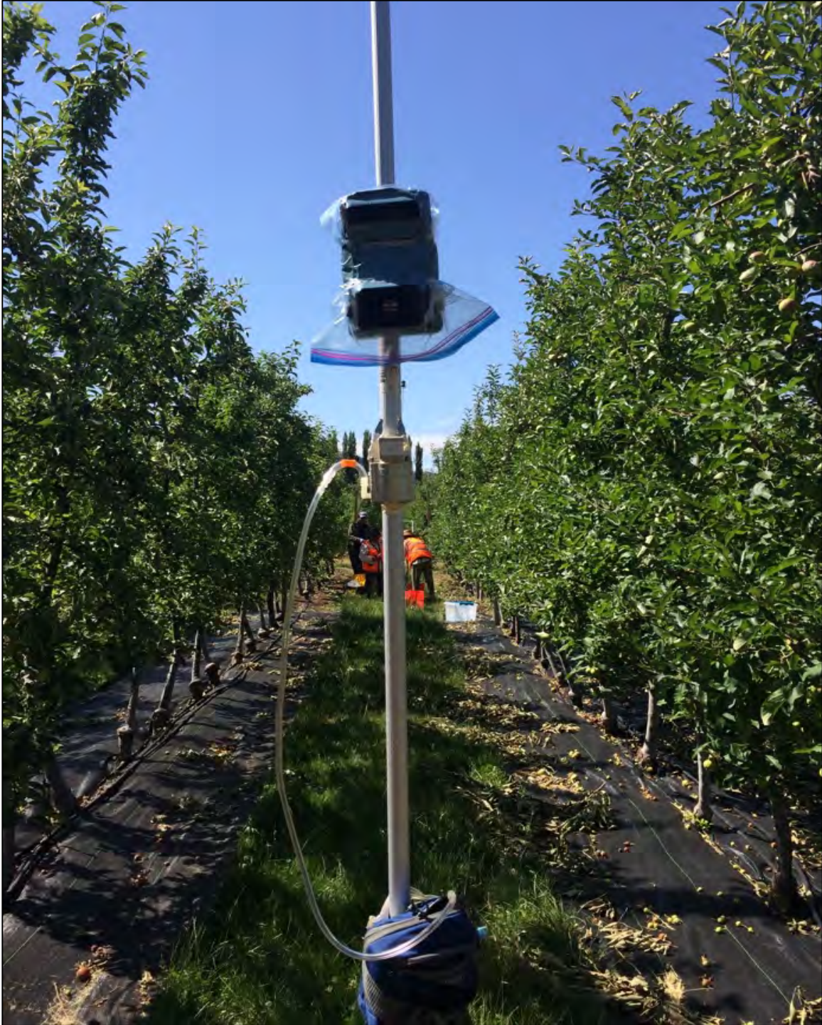
Figure 10. Dylos Particle Sampler at 2 Meters
