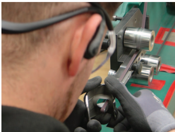
FIGURE 1. An employee polishes the inside of a square femoral implant with a thin band of sandpaper at the box polish station (photo by NIOSH).
