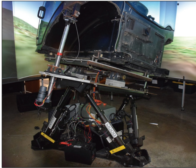
Figure 6. The motion system is comprised of two stages. The lower stage is an electrical, six-degrees-of-freedom Stewart platform (model 6DOF2000E-170122A, Moog, Inc.). On top of that, a custom-built, one-degree-of-freedom mechanism provides additional roll motion.
