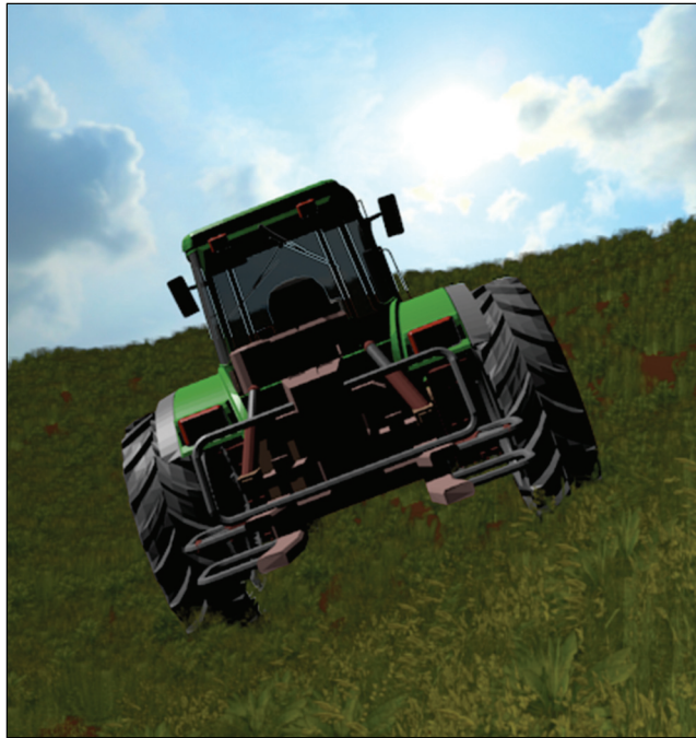
Figure 2. Tractors frequently operate at bank angles that are not encountered in other driving scenarios, and rollover events occur at roll angles beyond the normal motion capabilities of driving simulators.
