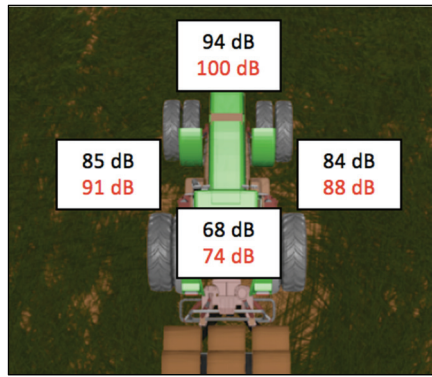
Figure 4. Noise level measurements (A-weightings) conducted on a T7-270 New Holland tractor at various engine speeds. Upper numbers (in black) are the amplitudes of typical noise, and lower numbers (in red) are the maximum noise levels to which drivers are exposed.
