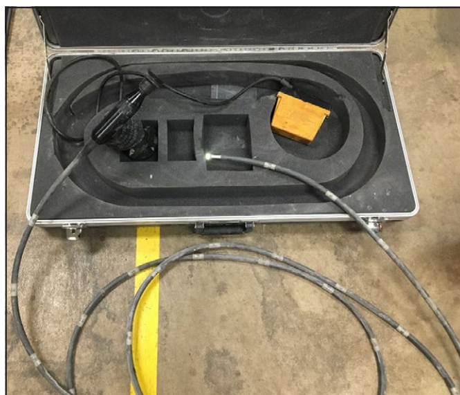
Figure 1. Fiberscope with a miner's cap light
