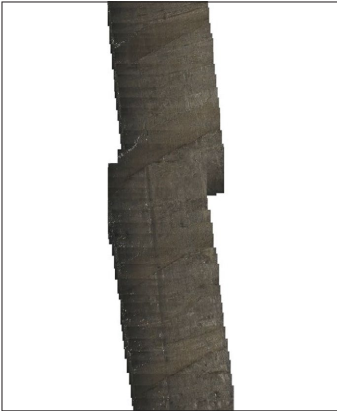
Figure 11. Multiple images stitched together from a continuous section of a borehole
