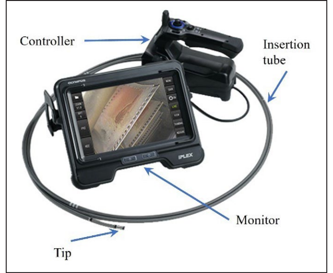
Figure 6. The side-view video scope used in this study
