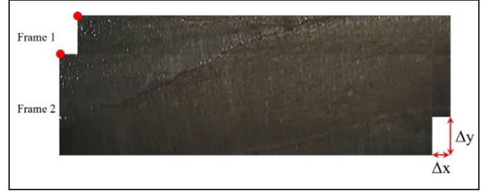
Figure 5. Offset calculation between two adjacent images
