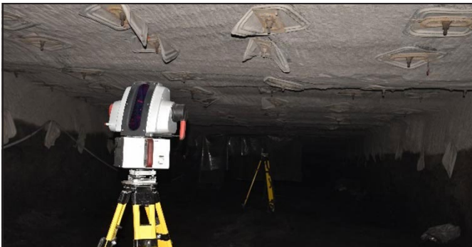
Figure 4. Monitoring entry deformation by LiDAR scanner before and after mineby
