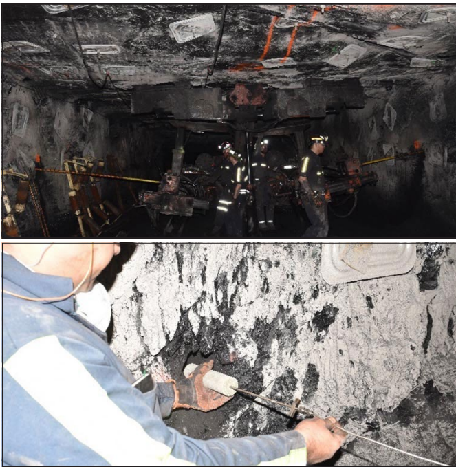
Figure 3. Drilling two 30-ft boreholes by a double-boom bolter (top) and installing BPCs with initial pressure set to 1,800 psi (bottom)
