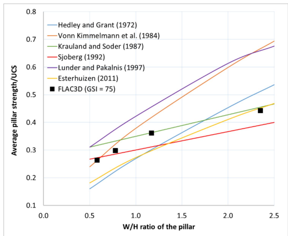
Fig. 3 Comparing the empirical pillar strength equations with FLAC3D model results
