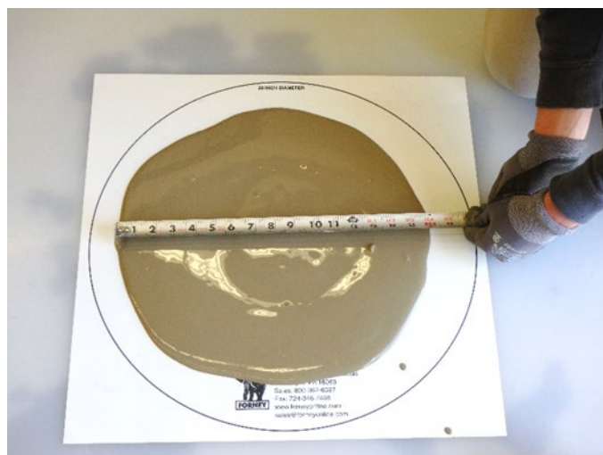
Fig. 5. Spread test for determining consistency of CPB mix.
