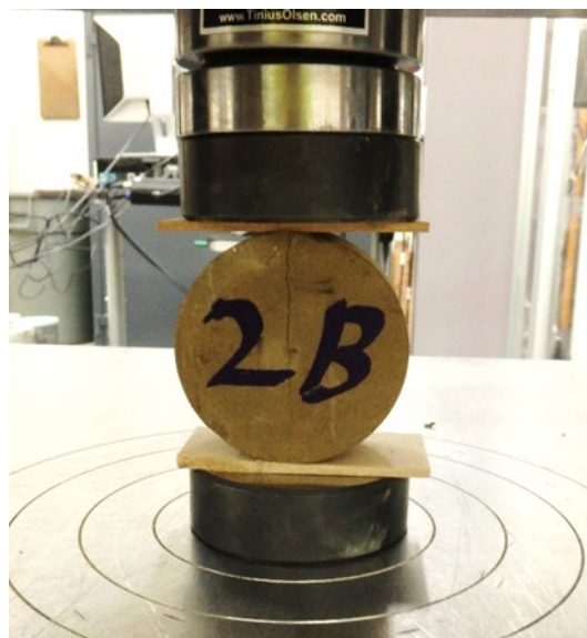
Fig. 10. Brazilian STS test with a disk-shaped CPB sample.
