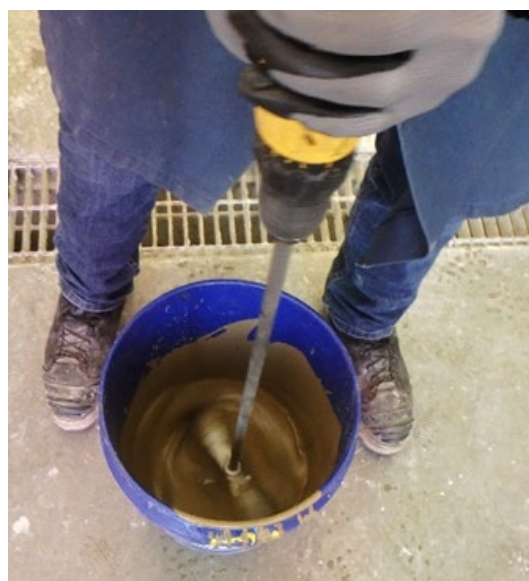
Fig. 6. Additional agitation of backfill mix during casting of CPB cylinders to prevent gravity separation of solids.
