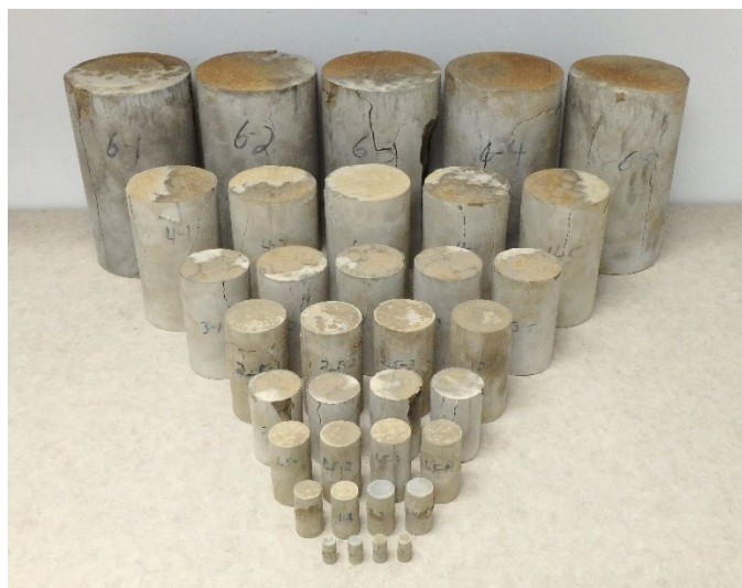
Fig. 12. Typical UCS test samples from the first test series ranging in size from 0.5×1.0 inch (13×25 mm) to 6×12 inches (150×300 mm).
