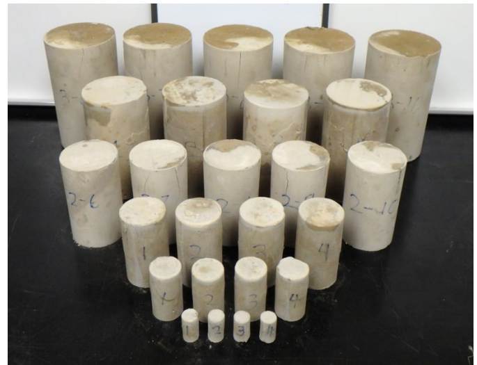
Fig. 16. Typical UCS test samples from the third test series ranging in size from 0.5×1.0 inch (13×25 mm) to 3×6 inches (75×150 mm).
