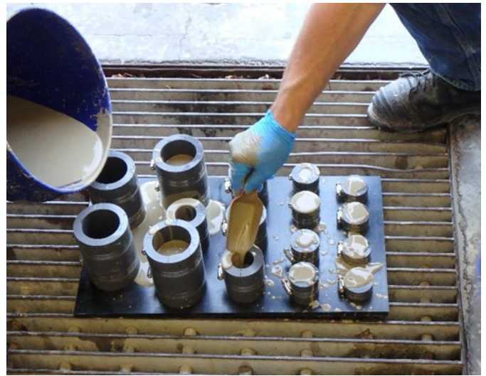
Fig. 4. Casting odd sized CPB samples using custom-made cylinder forms.
