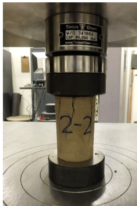
Fig. 9. UCS test with a 2×4-inch CPB sample.
