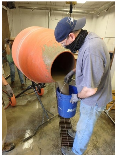
Fig. 3. Using a portable rotary mixer to prepare a CPB batch.
