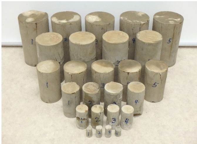
Fig. 14. Typical UCS test samples from the second test series ranging in size from 0.5×1.0 inch (13×25 mm) to 3×6 inches (75×150 mm).
