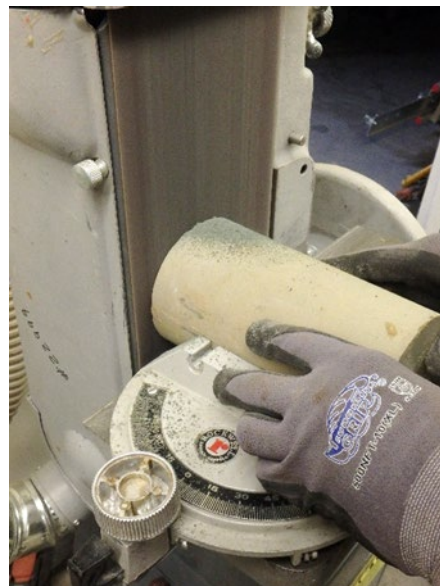
Fig. 8. Preparing the end of a CPB sample.
