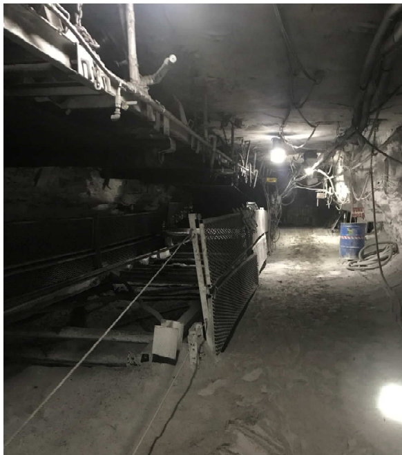
Figure 2: Coal conveyor belt with head end drive motor (out of view.)
