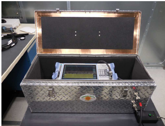
Figure 3: R&S FPL1000 placed in portable shielded enclosure.
