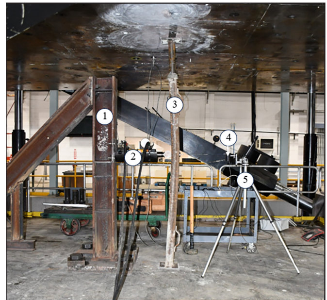
(1) Lateral loading fixture mounted on the floor of the MRS (2) Hydraulic loading ram (3) Tested Type-1 prop (4) String pot (5) Tripod
