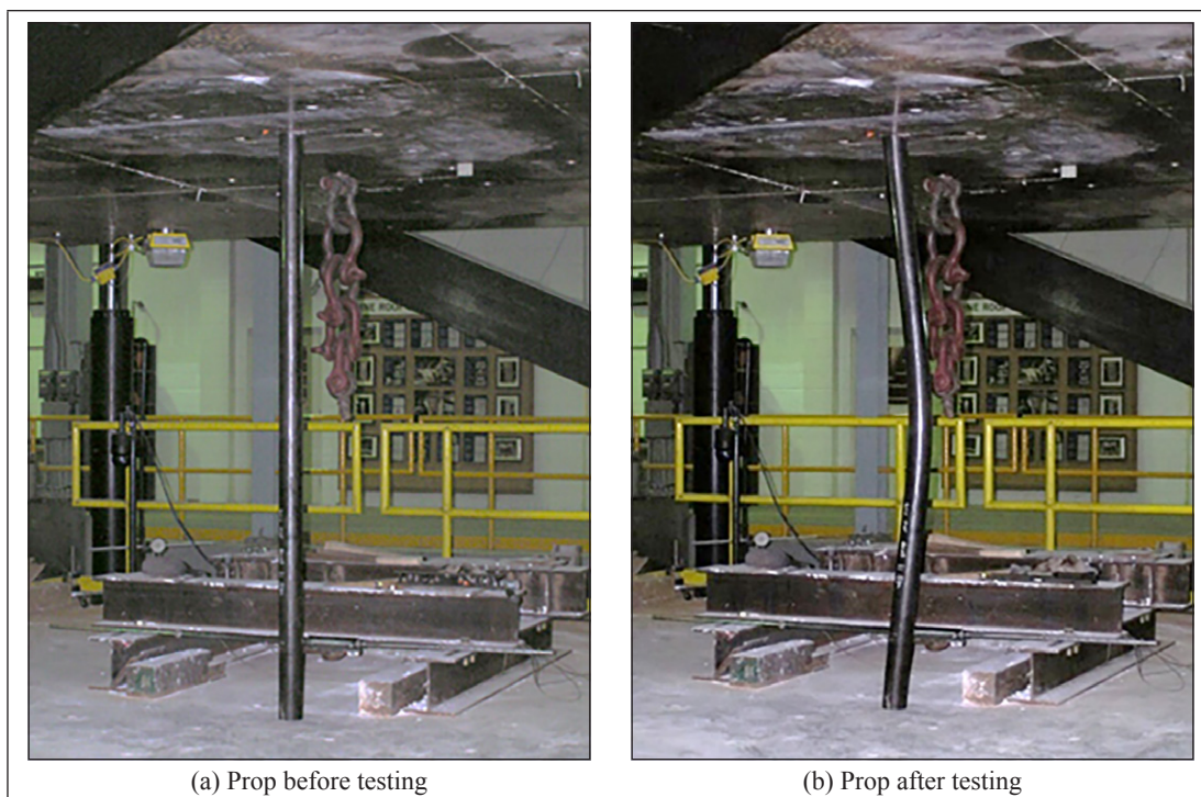
Figure 6. Type-2 prop (8-ft height) before and after experimental testing
