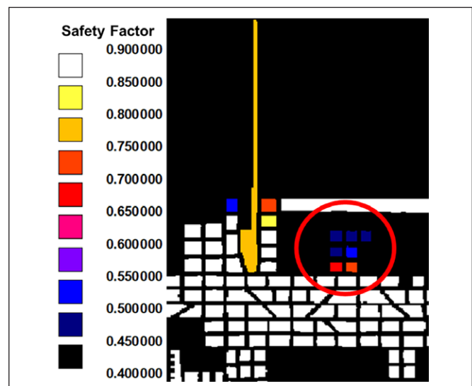
Figure 9. Pillar stress safety factors for the underlying Eagle seam after retreat mining the preceding panel
