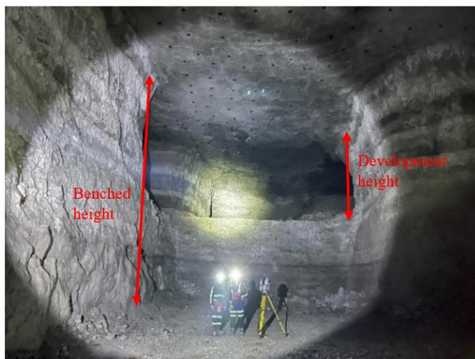
Figure 1: Development pillar height versus benched pillar height in an underground limestone mine.
