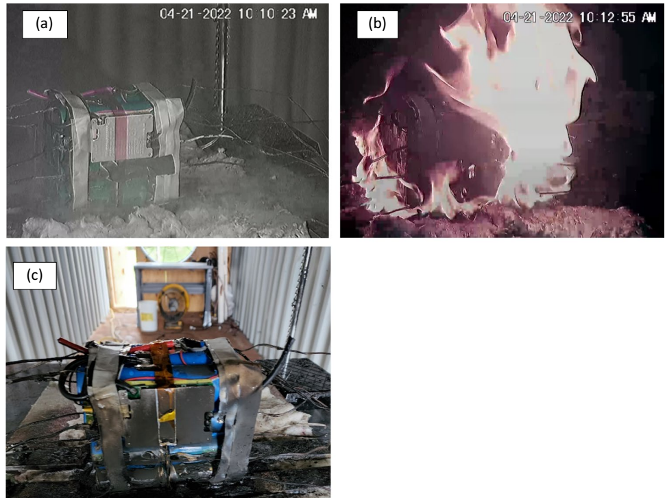
Fig. 6 Battery fire suppression using water mist. a Smoking of battery; b flame before suppression was on; c complete extinguishment
