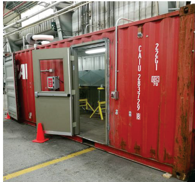
Fig. 1 The tests were conducted in the shipping container. The shipping container was modified to represent a refuge alternative or other confined space.
