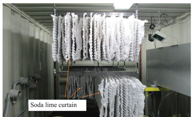
Fig. 6 The CO 2 scrubbing curtain, or soda lime curtain, was used as CO 2 mitigation to absorb the CO 2 generated during the test
