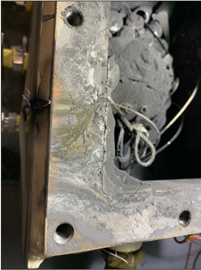
Figure 11. Escaping gasses etched a path through soot that accumulated in the cover joint
