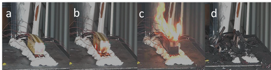
Fig. 1 Free burn: (a) smoke starts, (b) flame starts, (c) explosion and (d) burnout.
