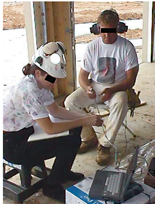
Figure 11 A NIOSH researcher conducting hearing protector fit-testing using a Real Ear Attenuation at Threshold (REAT)-based system at a construction job site. The worker listens to test signals through a set of large-volume headphones while the tester establishes hearing thresholds with and without the ear-plugs in place.
