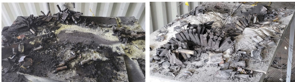
Figure 10. Scattered NMC cells after flame was out with (a) dry chemical system (left) and (b) Class D powder system (right).
