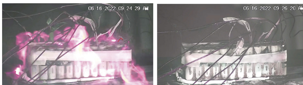
Figure 7. NMC battery fire suppression with water mist; (a) flame before suppression (left) and (b) flame out after water mist (right).
