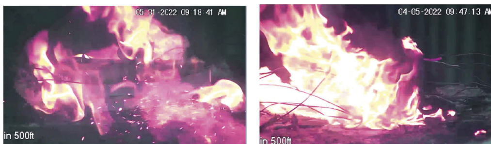
Figure 3. 12V battery pack free burn (a) NMC (left) and (b) LFP (right).
