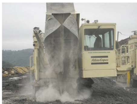
Figure 3. Dust generated during the lowering of the drill mast.
