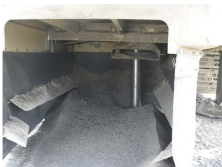
Figure 2. The buildup of drill cuttings on the air-blocking shelves.
