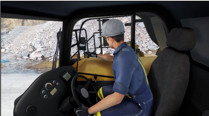
Figure 2. Still frame from video 1: "It's the Little Things," where the operator is reaching to close the door that popped open and is not wearing a seat belt.
