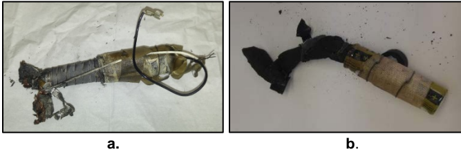
Figure 9. a) an LFP cell and b) an LTO cell after ejecting their contents during thermal runaway.
