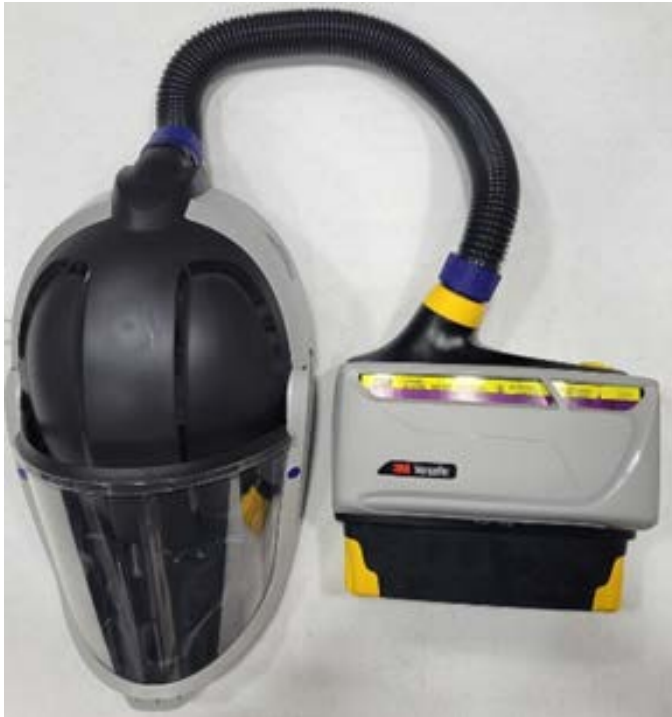
Figure 2. A picture of the 3M PAPR (Versaflo™ TR-801N) that NIOSH researchers evaluated in terms of its magnetic field emissions.
