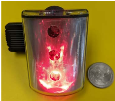
Figure 6. A picture of an MSHA-approved permissible lite tracker (Model 2004M) used in underground coal mines.
