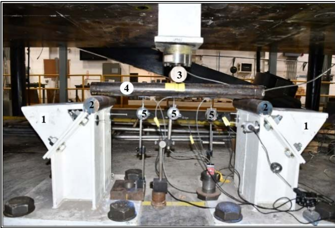
(1) Reaction frames (2) Roller supports (3) Loading roller (4) Inner tube specimen (5) Displacement gauges
