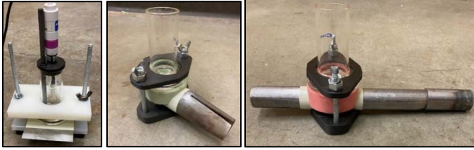
Figure 2. Modified paint cells for electrochemical testing.
