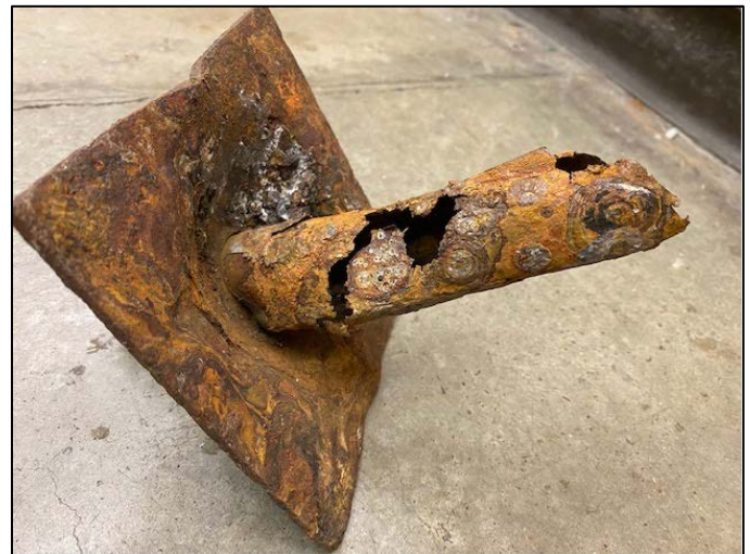
Figure 1. Failed corroded rockbolt from a mine in this study.
