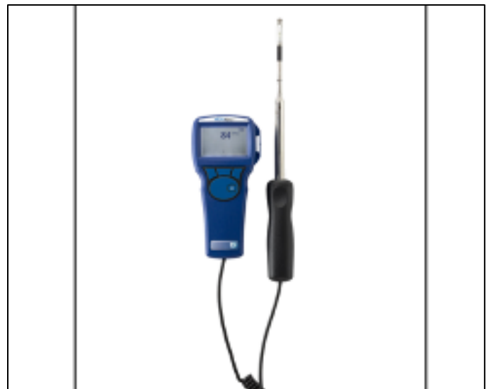
Figure 1. TSI Velocicalc 9535 air meter used for low-velocity, point-based measurements.
