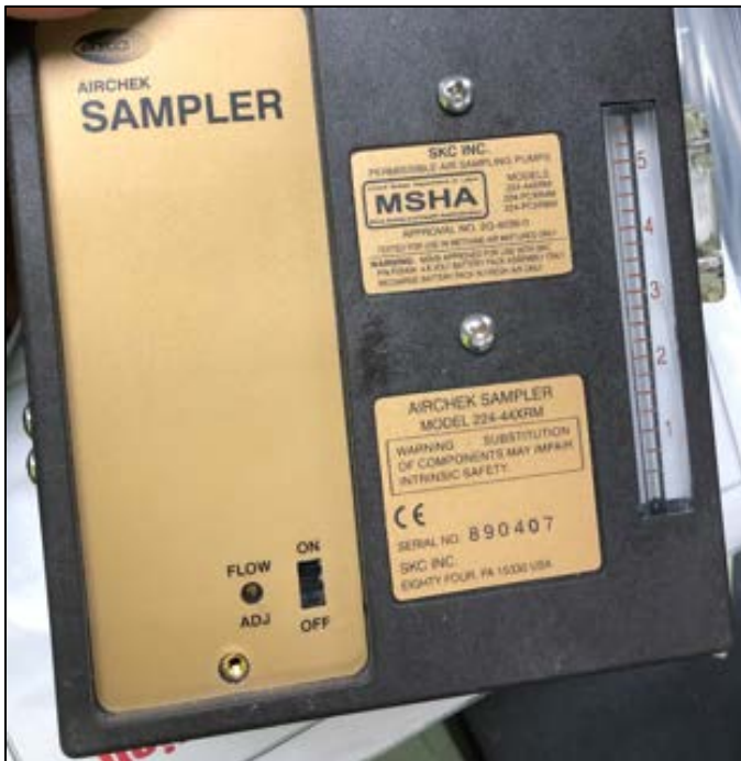
Figure 2. Pumps for DPM sampling using the NIOSH 5040 method.
