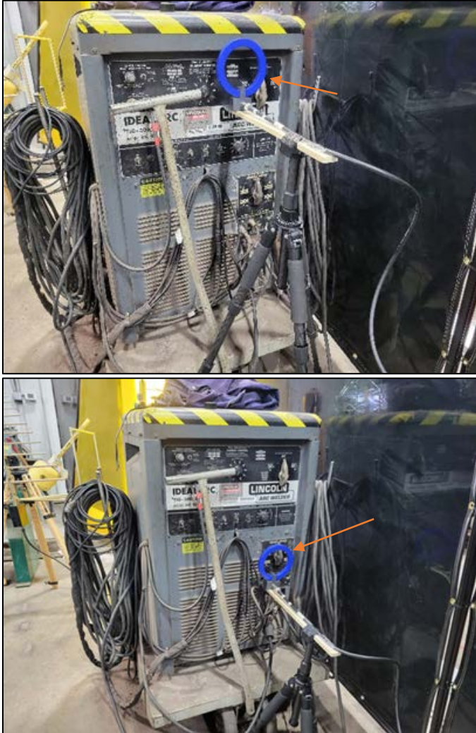
Figure 10. The B-field was measured at the upper and lower portions of the front panel of the welder while cable was coiled nearby.
