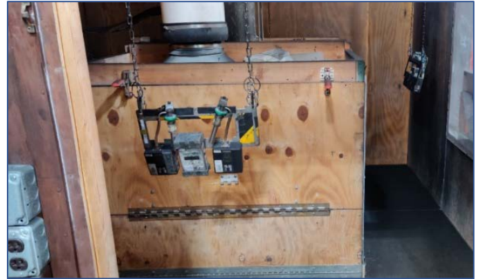
Figure 2. A sampling package consisting of a pDR-1000 and two gravimetric samplers used in the air-cleaning fan evaluation test.
