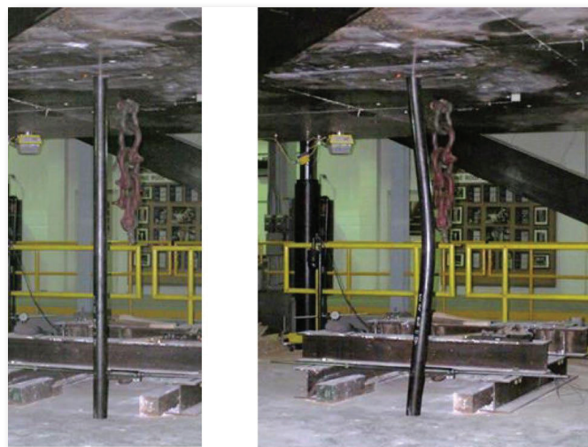
Fig. 1 Vertical load capacity test setup for steel props.
