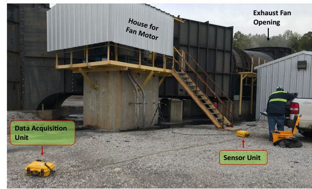
Fig. 2 ANDAU system was placed near a ventilation fan for an underground coal mine to survey the ambient EM noise in the fan area
