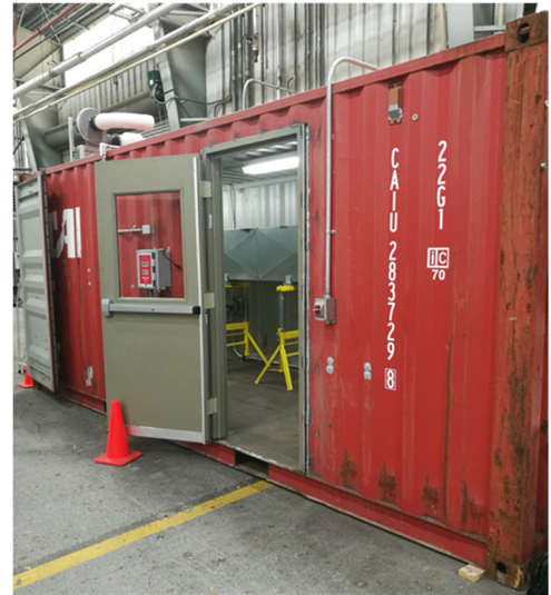
Figure 1. The tests were conducted in the shipping container. The shipping container was modified to represent a refuge alternative or other confined space.
