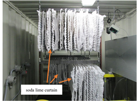
Figure 6. The CO 2 scrubbing curtain, or soda lime curtain, was used as CO 2 mitigation to absorb the CO 2 generated during the test.
