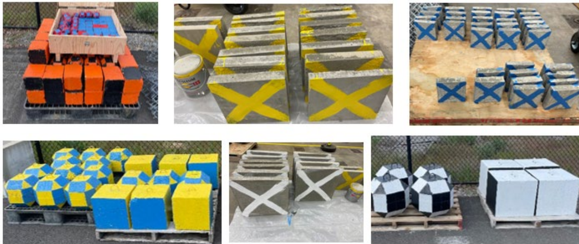
Figure 2. Photos of synthetic rocks colored to distinguish size and shape during post testing analysis
