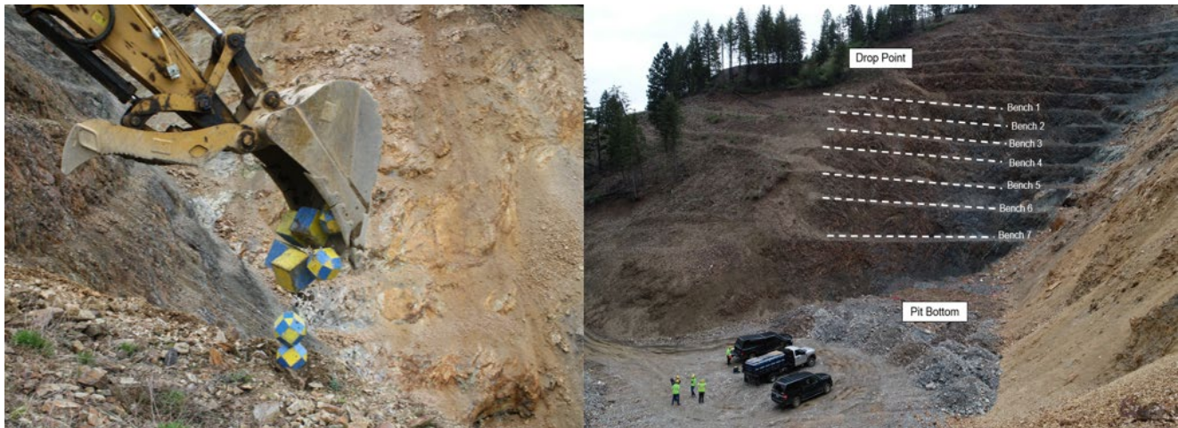
Figure 4. CAT 336 used to cast synthetic rocks down the slope (left) and the view from observation area (right).
