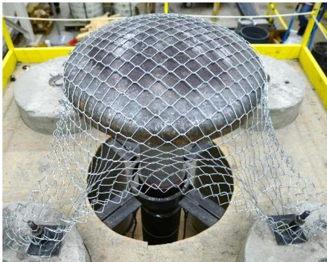
Fig. 3. Post-test photo of a chain-link test sample, maximum sample displacement.
