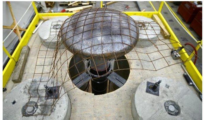
Fig. 5. Post-test photo welded wire test sample, maximum sample displacement.
