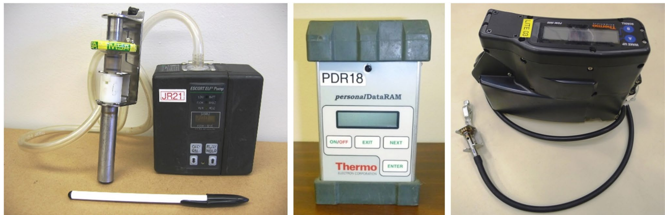
Fig. 6 The samplers used during the study; gravimetric (left), instantaneous (middle), and CPDM (right)
