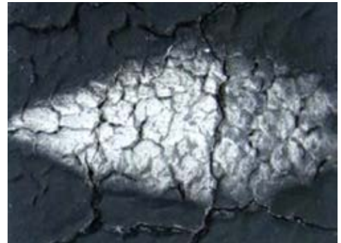
A blast of air disperse a layer of water-resistant coal dust on top of moisture-absorbing non-dispersible rock dust.
