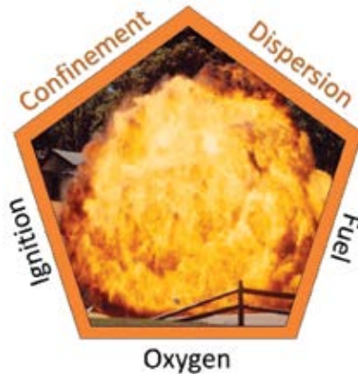
The dust explosion pentagon showing the five required components for a dust explosion.
