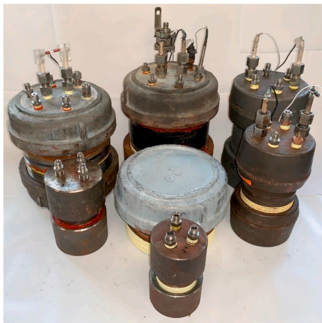
Fig. 1. Canisters provided varying amounts of free space around enclosed Li-ion cells.
