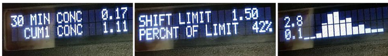
Fig. 4 Information displayed by the PDM3700. The first screen shows 30-minute and cumulative dust concentrations (left), with the second screen showing the shift dust limit and the percentage of the
