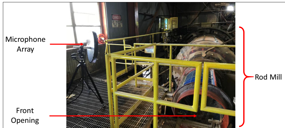
Fig. 15 Rod mill used in the processing building, with the microphone array on the left side
