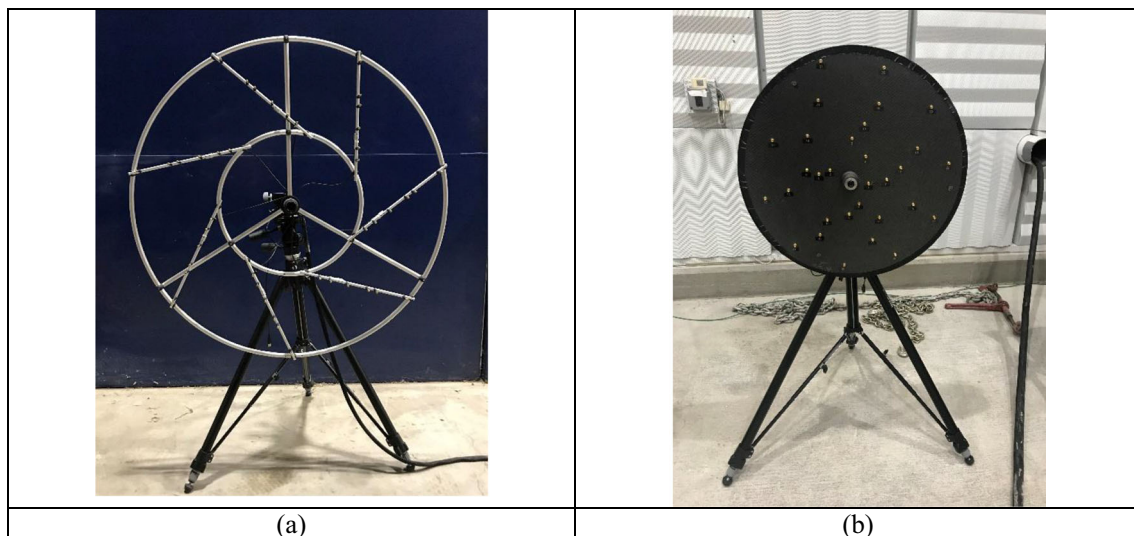
Fig. 2 Microphone phased arrays used for this study
