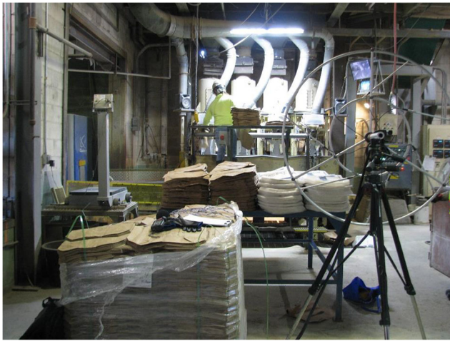
Fig. 3 Automatic bagging machine and operator in the background, with the microphone array in the foreground
