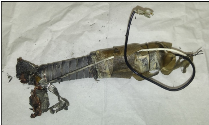
Figure 8. LFP cell after ejecting its contents during one of the elevated peak pressure tests.
