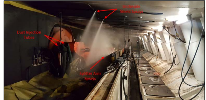
Figure 1. NIOSH longwall gallery showing the dust injection system located near the shearer drum, with splitter arm and underside shield sprays in operation without dust injection.
